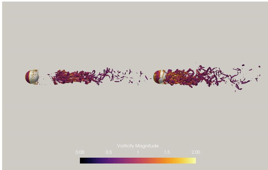
Figure 1: Visualization of the near wake region with iso-surfaces of Q-criterion colored by vorticity magnitude.
