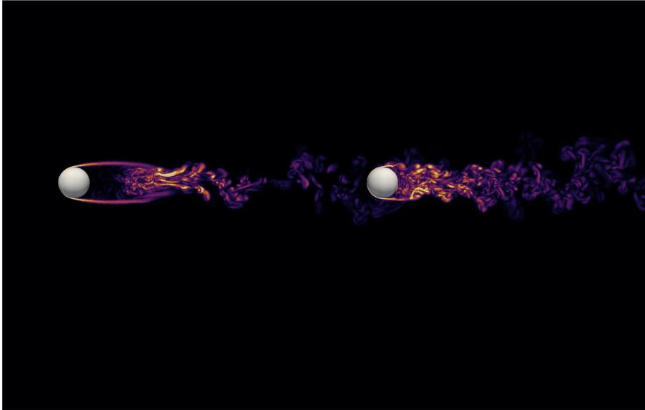
Figure 2: Visualization of the near wake region with vorticity magnitude on a plane passing through the sphere centers.
