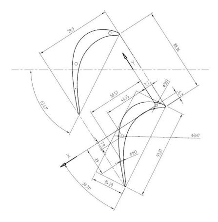
The geometry of the T106C cascade is shown above. The blade description is available as IGES/step CAD file constructed from the coordinates provided by R. Stieger<sup>2</sup>. A single blade is to be computed, assuming pitchwise and spanwise periodicity, corresponding to 10% of the axial chord for the latter.
